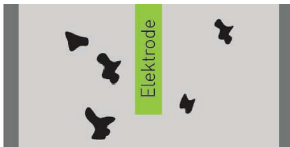
1. Fine dust particles flow through the exhaust duct with the exhaust air.
